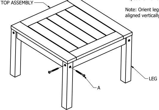
Attach leg to table top using (2) A bolts. Repeat for remaining (3) legs.
